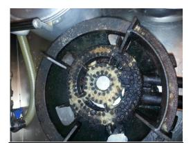
Remove food particles from the burner regularly. Also to ensure there are no blockages to the gas outflow.
