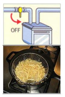
Ensure that main gas and stove valves are switched off, before tenants leave the premise. The valve handle should be seated perpendicular to the service pipe (i.e. 90 degrees). Remember to <u>switch off the cooking stove</u> to avoid unnecessary extended heating of cooking oil before leaving cooking area.
