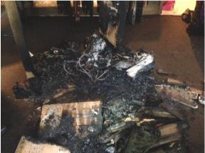
Fire at T2 on 11 Oct 2014. Investigation found Fire at T3 on 13 Oct 2014. Investigation determined that the origin of the fire was from the electrical wiring below a carpet where the display cabinet was placed.
