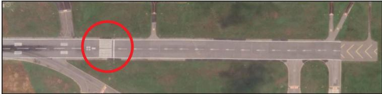
Runway 20R has a displaced threshold, which is a threshold located a certain distance after the start of the physical runway. The area leading up to the displaced threshold is marked by white arrows. A displaced threshold is necessary because of the presence of obstacles such as water bodies or buildings in a landing aircraft's approach path.
