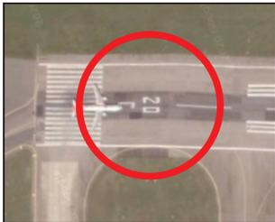
Runway designators are white markings painted on each end of the runway, indicating the compass heading of the runway centerline.
