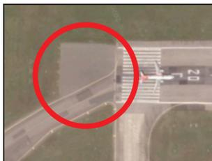
An area beyond the runway which can be used for deceleration of aircraft in the event of a rejected take-off.
