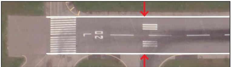
Runway edge markings are continuous white stripes near the edges of the runway pavement.
