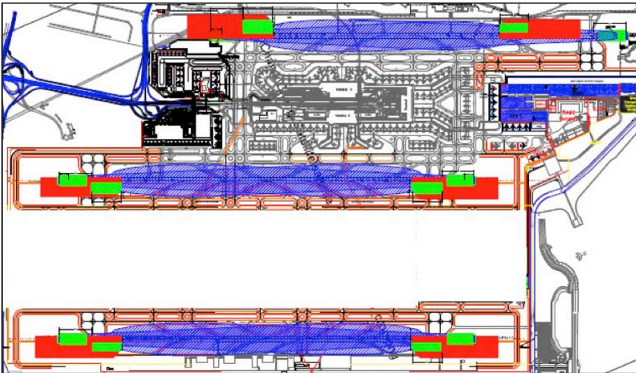
CSA (indicated in red and green above) are areas where the presence of vehicles may interfere with signals required by pilots for precision approach landings. Vehicles must stay clear of CSA. To enter CSA, permission must be sought from ATC.
